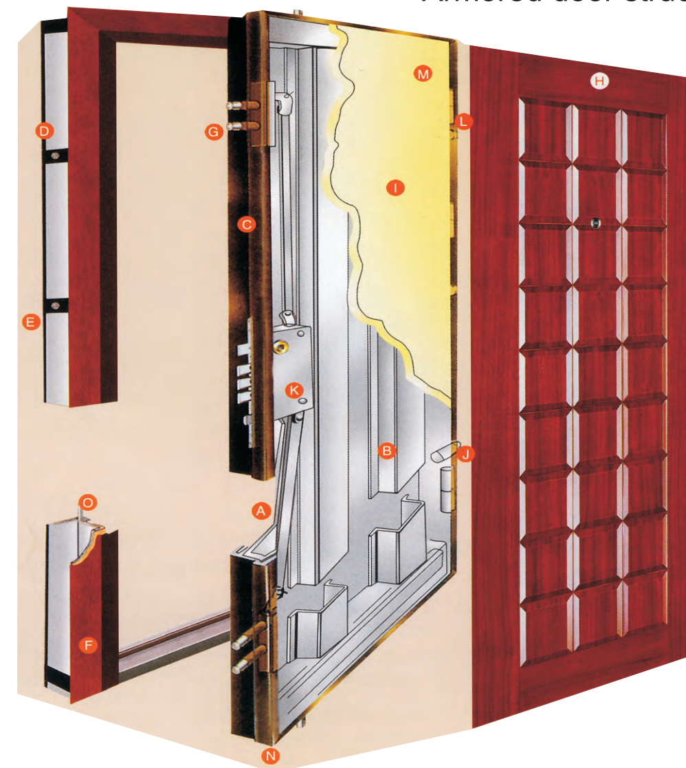
Armored door structure
