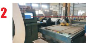
Carving pattern: Input the required pattern into the automatic carving machine to guarantee the high efficiency and accuracy.
