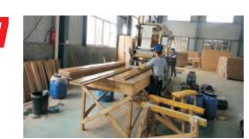
Laminating the film on the door frame.
