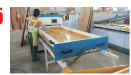
Laminating with PVC film by the machine.
