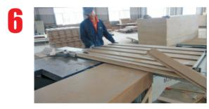
Assembling the door frame: cutting the board based on the customized size and press them.
