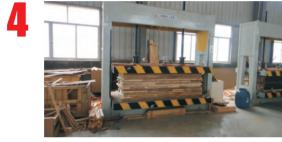
Assembling the fir wood and MDF board cold Pressing: Glue the melamine boards on both sides, to basic strong structure of door leaf. do cold pressing to make sure permanent stability.
